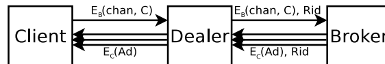
Figure 3: Message exchange for pub-sub ad dissemination. E_x(M) represents the encryption of message M under key x . B is the public key of the broker. C is a symmetric key generated by the client for only this subscription.
